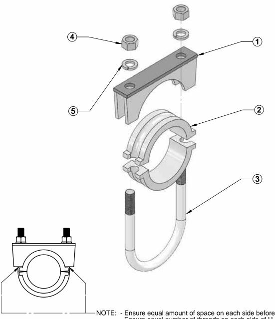
NOTE: - Ensure equal amount of space on each side before tightening U-Bolts .
